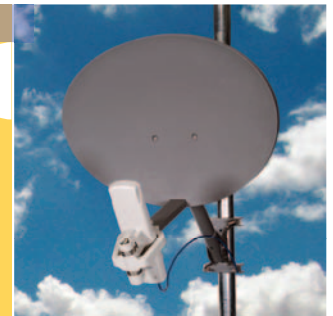
Backhaul with Passive Reflector
